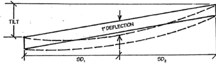
The **Inflection Point** is the location in the foundation where the direction of curvature changes. Refer to standard structural texts for elaboration of this term.
