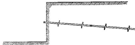
Step 2 - Install upper tier of soil screws.
