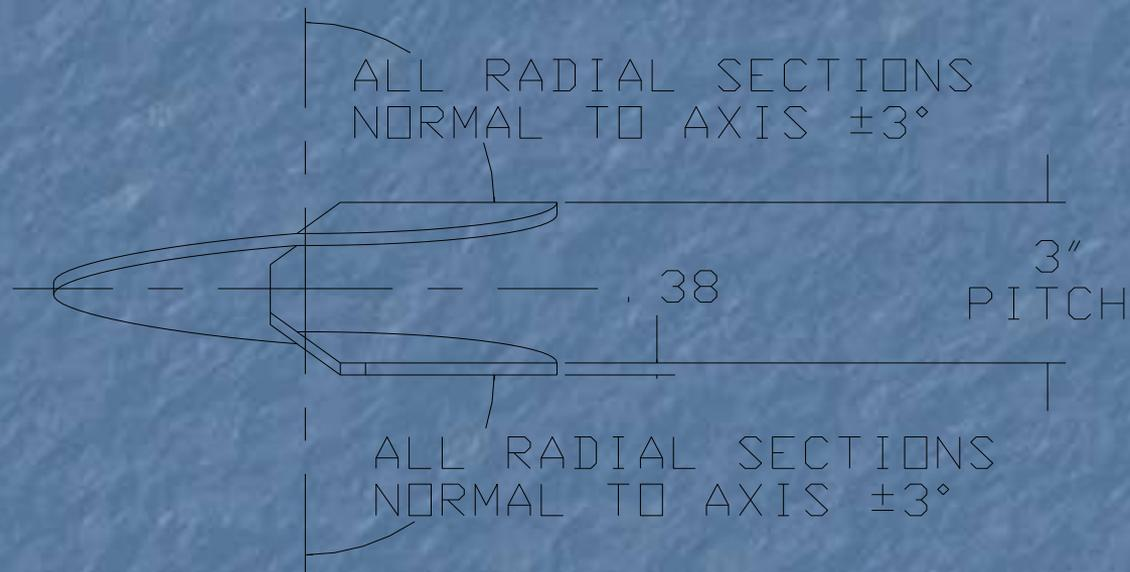
**Helix formed by matching metal die so that soil disturbance is minimized.**
