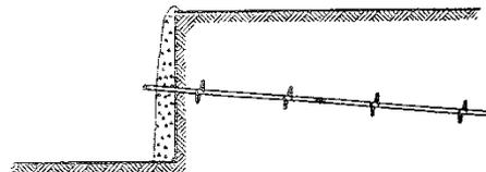
Step 3 - Install drainage strips, reinforcing steel and anchor plates, and apply initial shotcrete layer.
