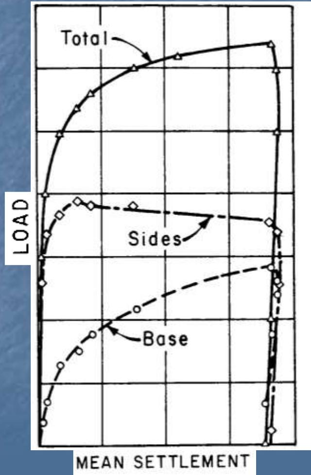
Maximum side resistance (friction) is mobilized after downward displacement of from 0.5 to greater than 3 percent of the shaft (grout column) diameter, with a mean of approximately 2 percent [Reese, Wright (1977)].
