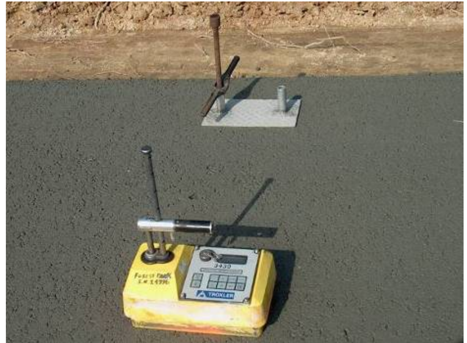
Nuclear Gauge - ASTM C1040 [Direct Transmission]
